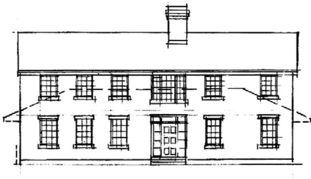
The Historical Conversion approach used in putting a second storey addition on the same 1970s ranch house.
