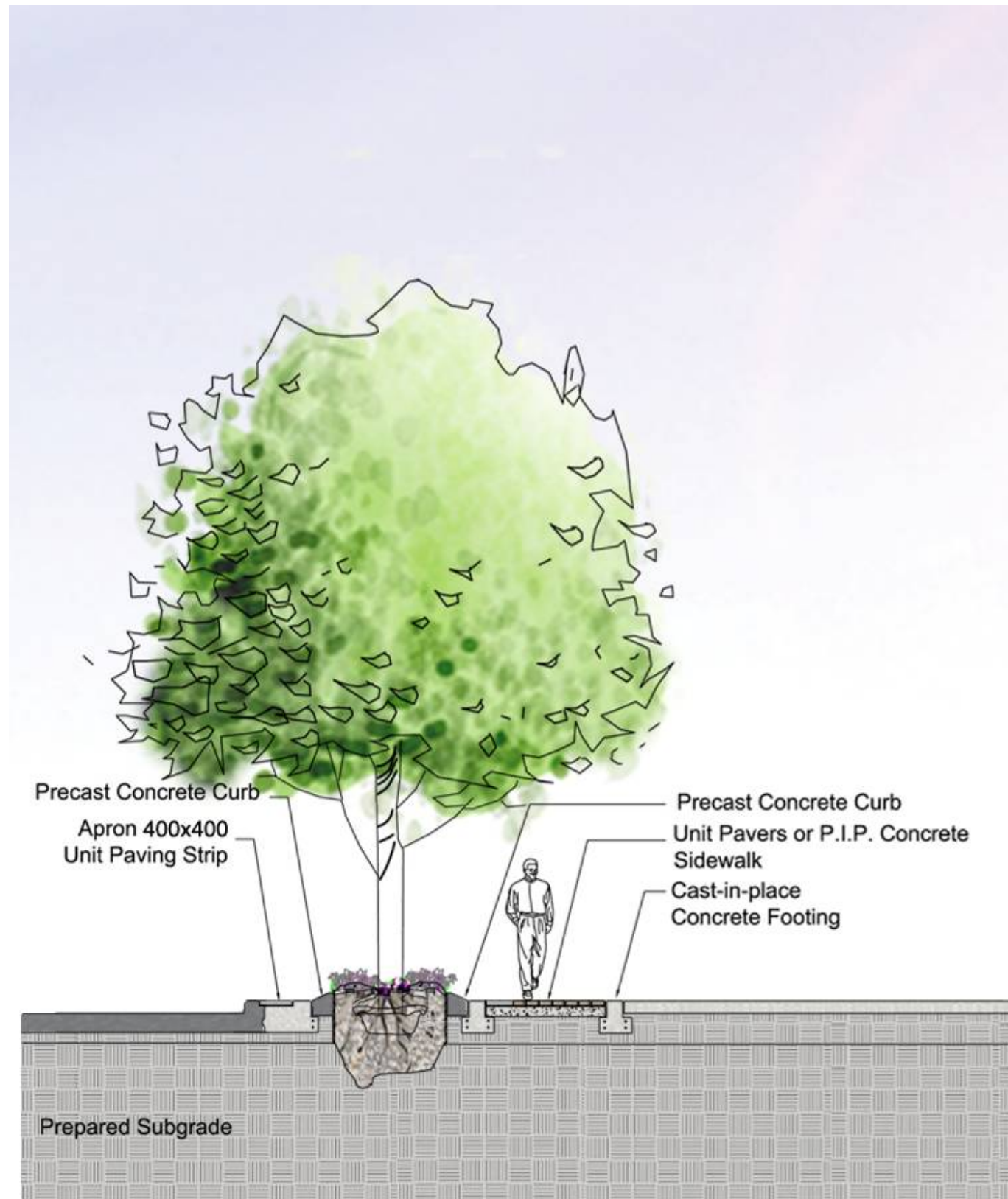
Figure 46: Typical Streetscape Detail - Special Character Road
