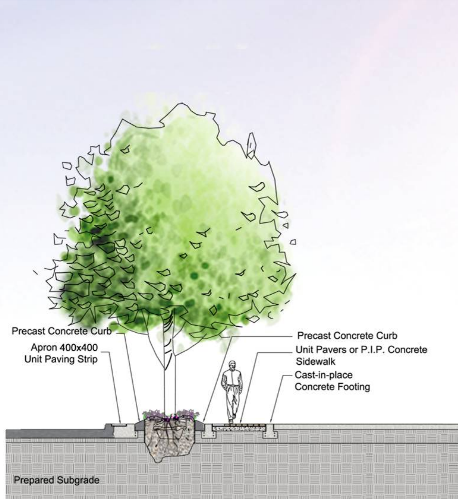
Figure 45: Typical Streetscape Detail - Local Road
