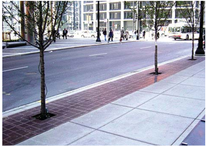
Figure 4.2: Tree grating that can sustain increased surface traffic
